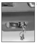
Open the hood and unwrap the electrical cord. The cord is located on the driver's side of the vehicle near the front recovery loop. 3. Plug it into a normal, grounded 110-volt AC outlet.
